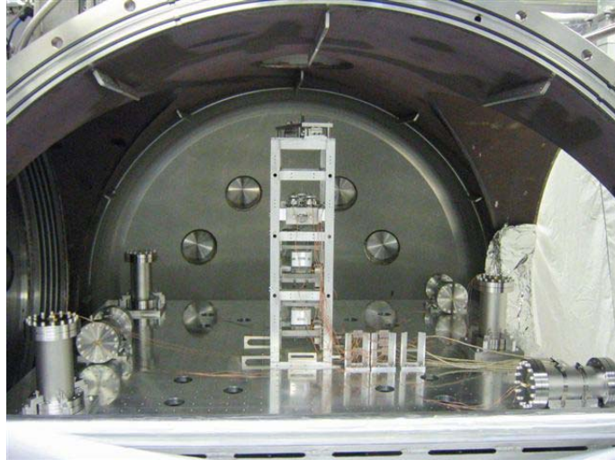
Ham optical table with pendulum and geophones installed
