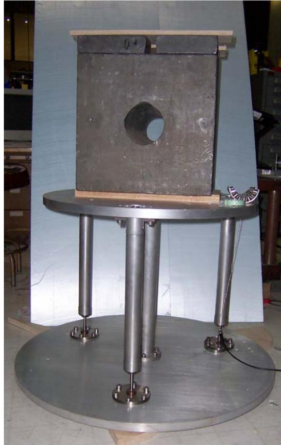
Figure 7: Small IP leg test setup (without counterweights) design and photo. The lead cube is a 500 Kg block (2/3 nominal load). Visible on the right of the block is one of the magnetic dampers to neutralize the first leg resonance. The central leg is a safety stop.
