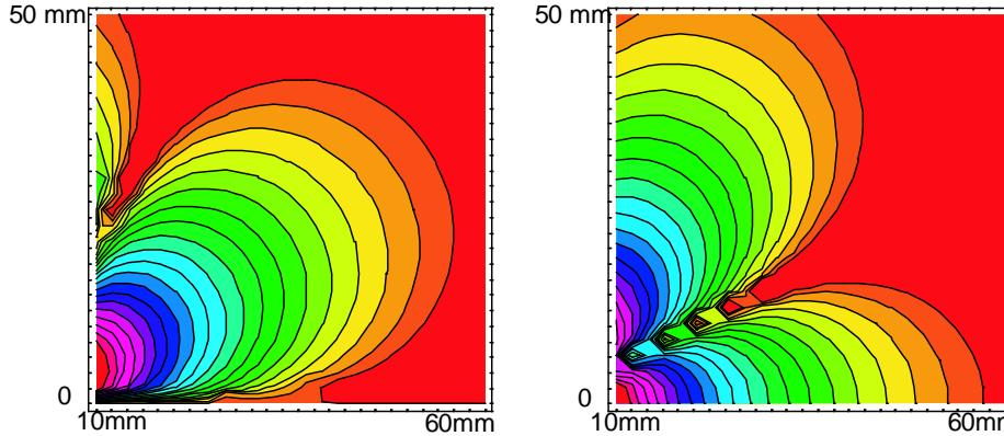
There are several field gradient (force) components that can be calculated. Depending on the geometry of the problem one or other will be more important. All are less than 1 mN (red) when the spacing in the (projection on to the) plane of the ECD magnet exceeds 60 mm, for any interesting position of the OSEM magnets out of the plane. Two examples of force as a function of position are shown with the ECD unit at 0,0. The contours are logarithmic at 1/6th decade intervals
