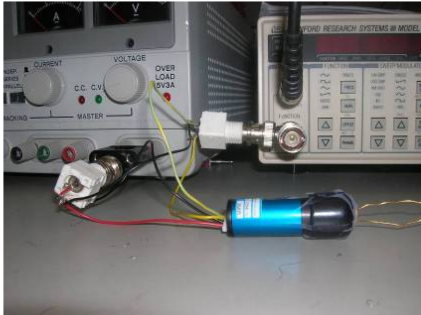
Figure 1.3.1.1: a picture of the laser connected to the photodiode
