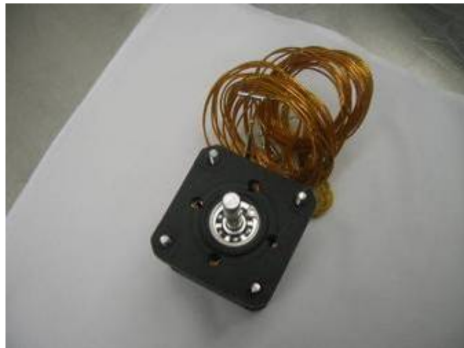
Figure 1.2.6: a photograph of the stepping motor which may replace the tuning mass of the suspension system for Advanced LIGO
