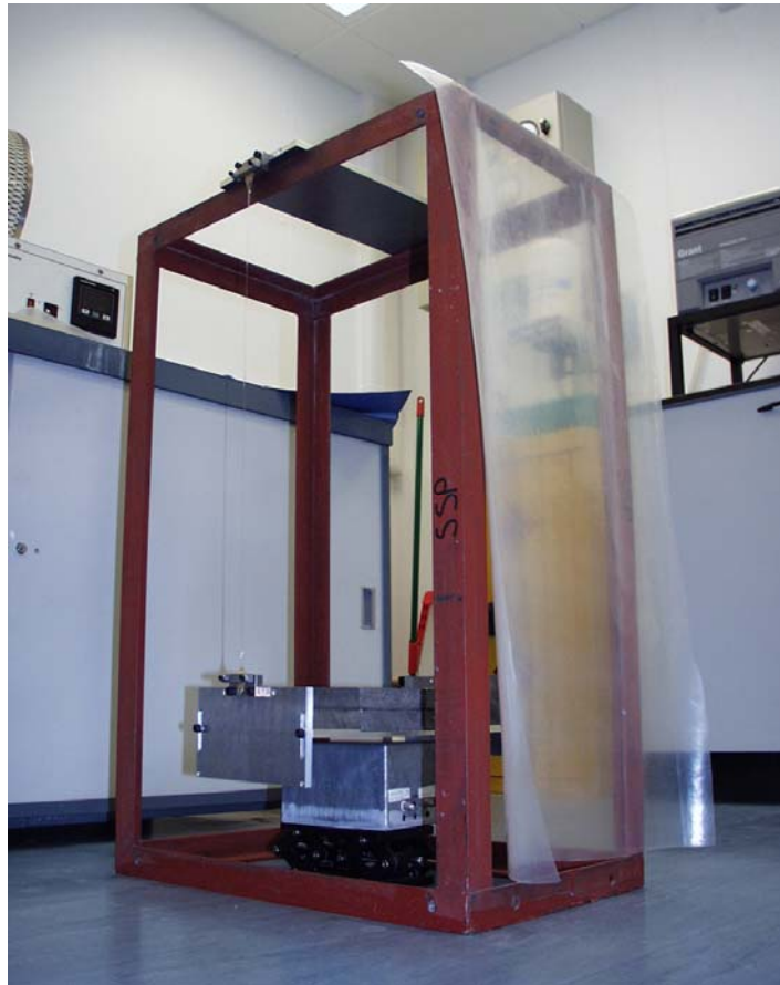
Figure 7 Two fibre 20kg test suspension
