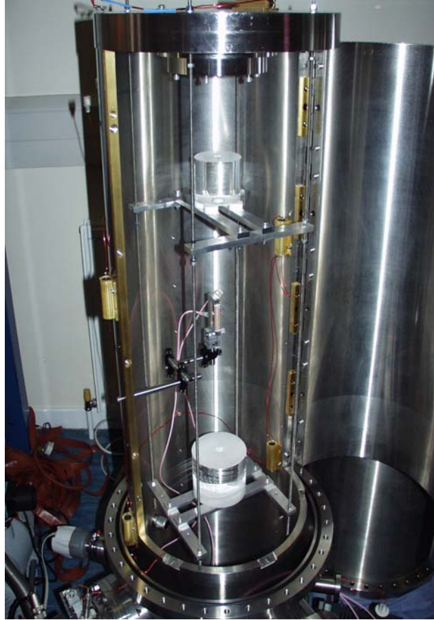
Figure 8 One of the mechanical loss measuring facilities, with ribbon fibre being tested
