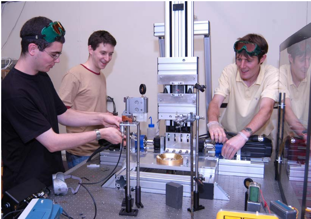
Figure 2 Development work being carried out on the CO 2 laser based pulling machine
