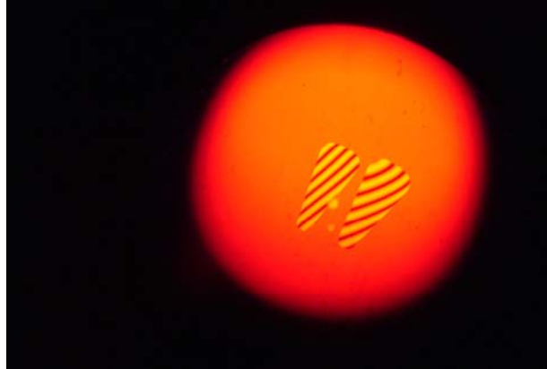
Figure 2. Interferogram indicating flatness of 'as received' Suprasil 2 'ears' – one supplied by Vendor 'A' (left) and one from Vendor 'B' (right). The Vendor 'B' ear flatness is considerably poorer.
