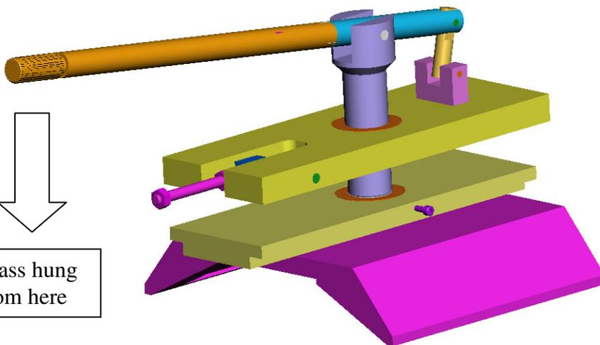
A longer arm can now be screwed into the lever arm, and a mass can be hung from it, out away from the test mass
