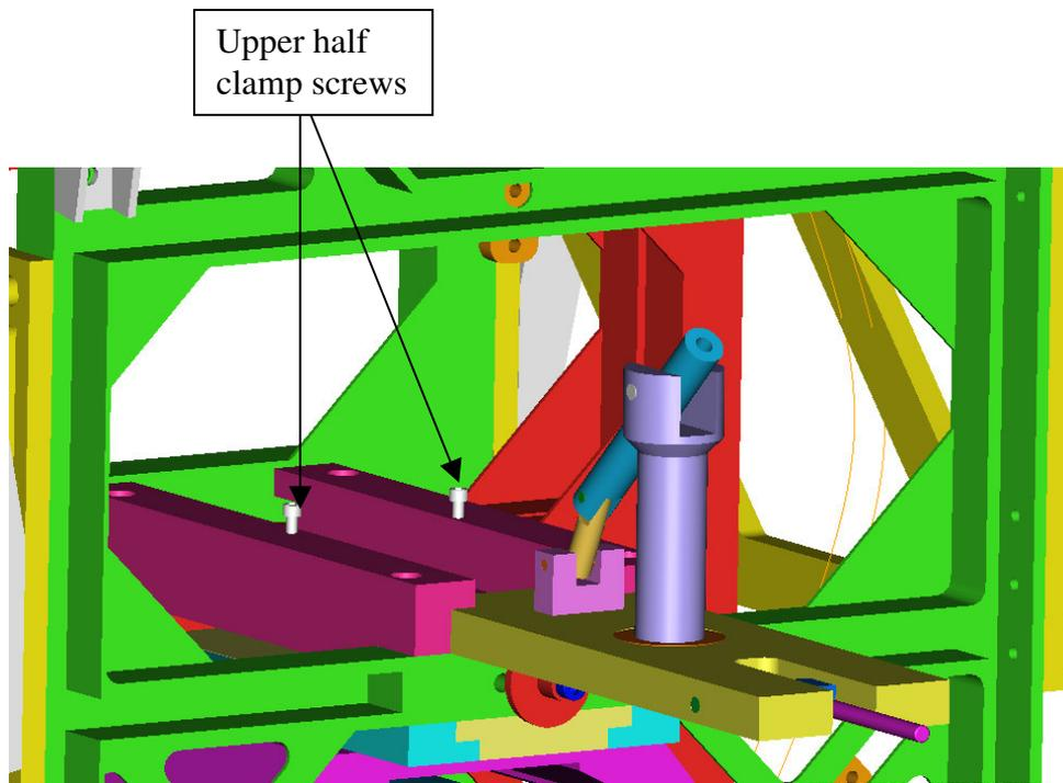
The lower locking piece can now be rotated through 180 degrees, out of the path of the lower part of the clamp, which can then be slid out of the structure
