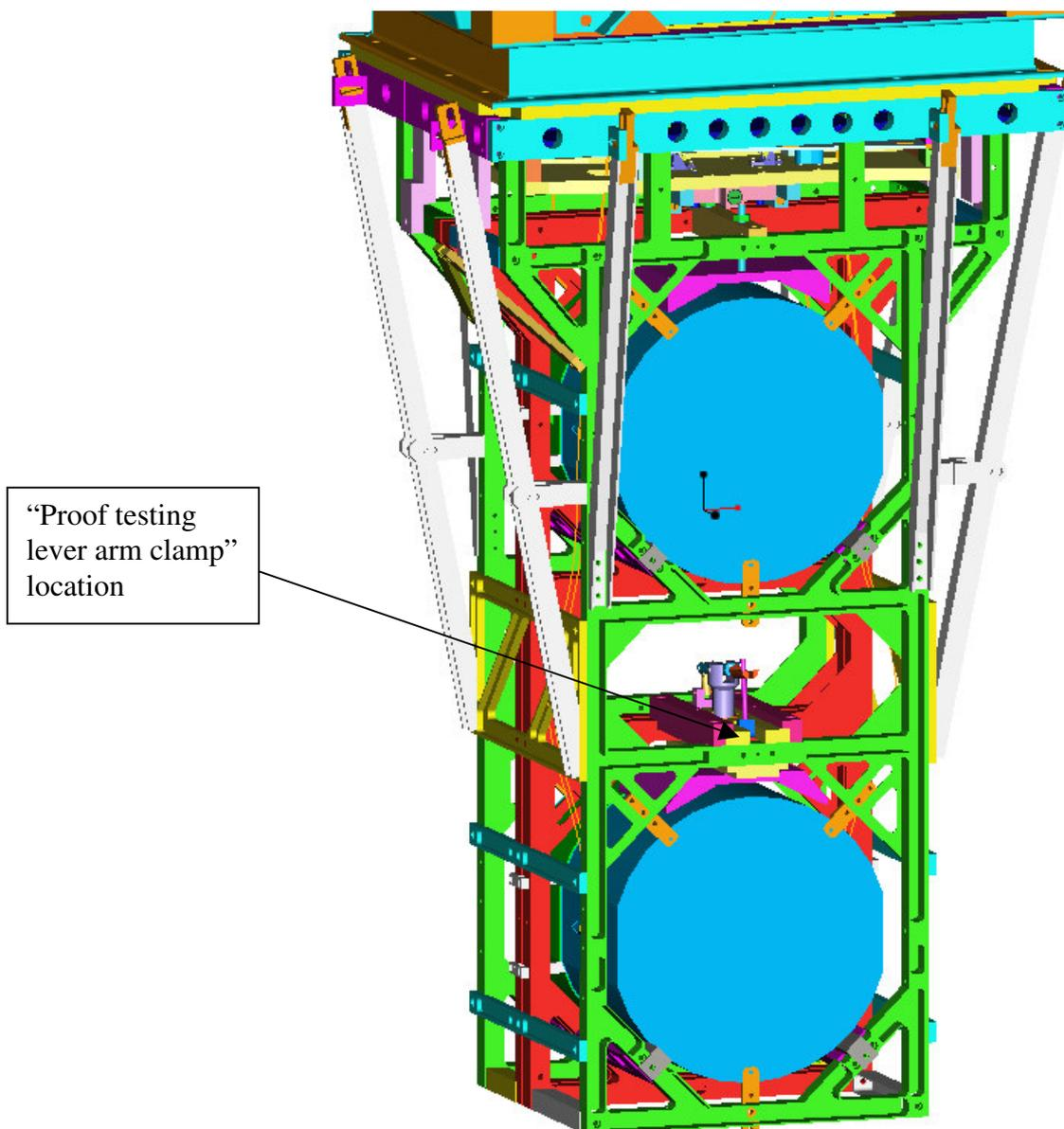
The clamp is mounted to the lower structure on “sliders”, which are bolted to the horizontal struts above the test mass. The sliders allow the variable load clamp to be added to, and removed from the lower structure without the risk of damaging the test mass or ribbons.
