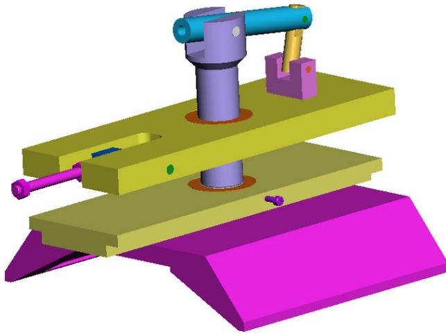
The clamp is raised to its full height, and the clamp locking screw is tightened; thus the clamp is held in place above the test mass.
