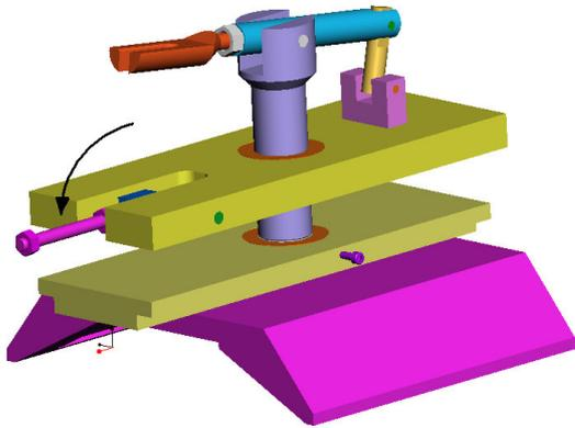
The jacking nut is released, and the threaded bar is rotated on its pivot pin, following the arrow, until it is resting on the horizontal member of the lower structure.
