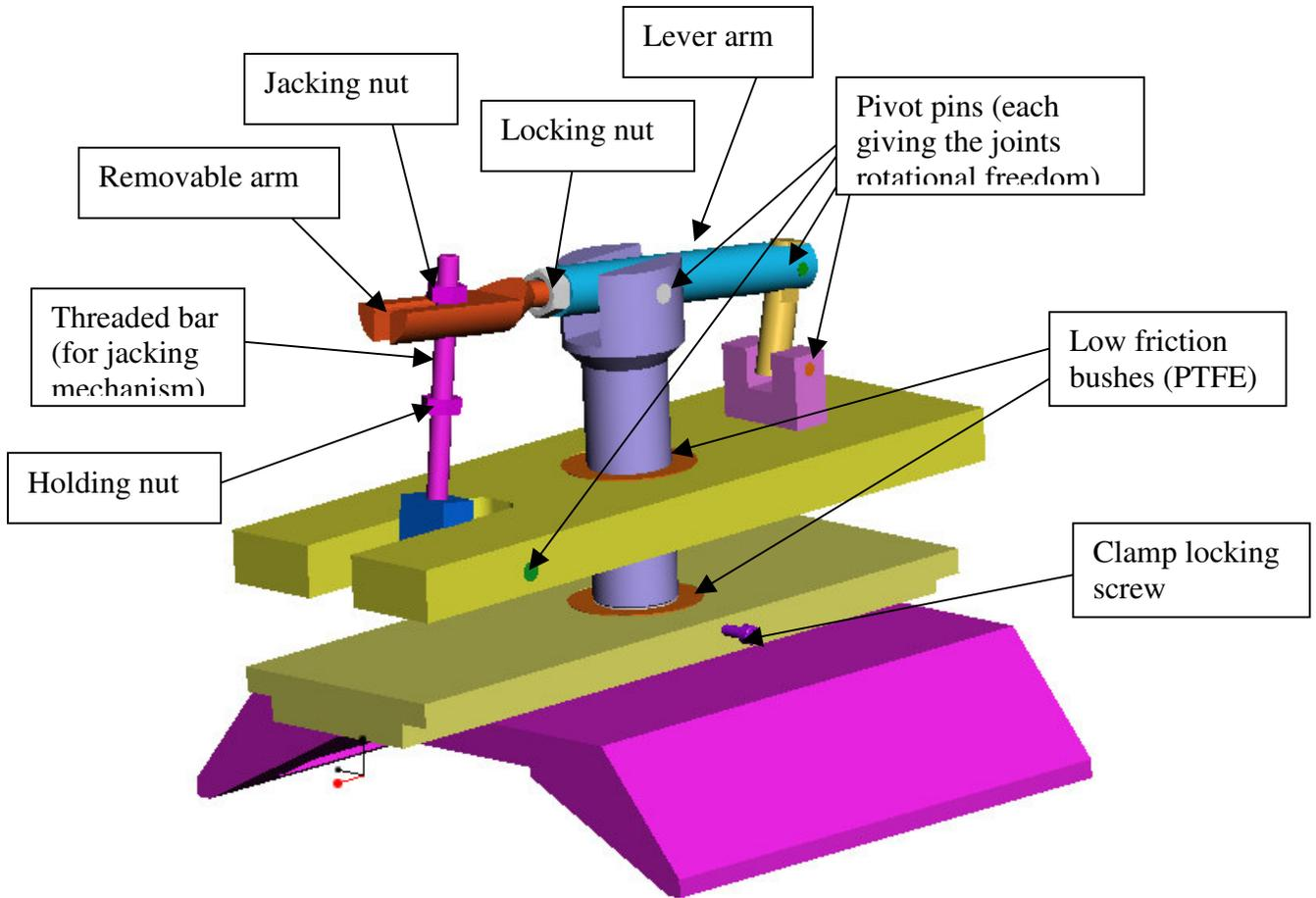
As the jacking nut is rotated clockwise, the piston is pushed downward through the low friction bushes, and the clamp jaw exerts pressure on the mass. When the clamping force is not needed, the clamp jaw can be held high up, away from the mass by slackening off the jacking nut, raising the removable arm up to its top position, and either tightening the clamp locking screw, or locking the holding nut up, against the removable arm.
