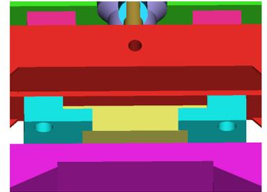
The “clamping jaw” can be locked in place above the test mass, and used to harbour the safety stops (not shown in the model)
