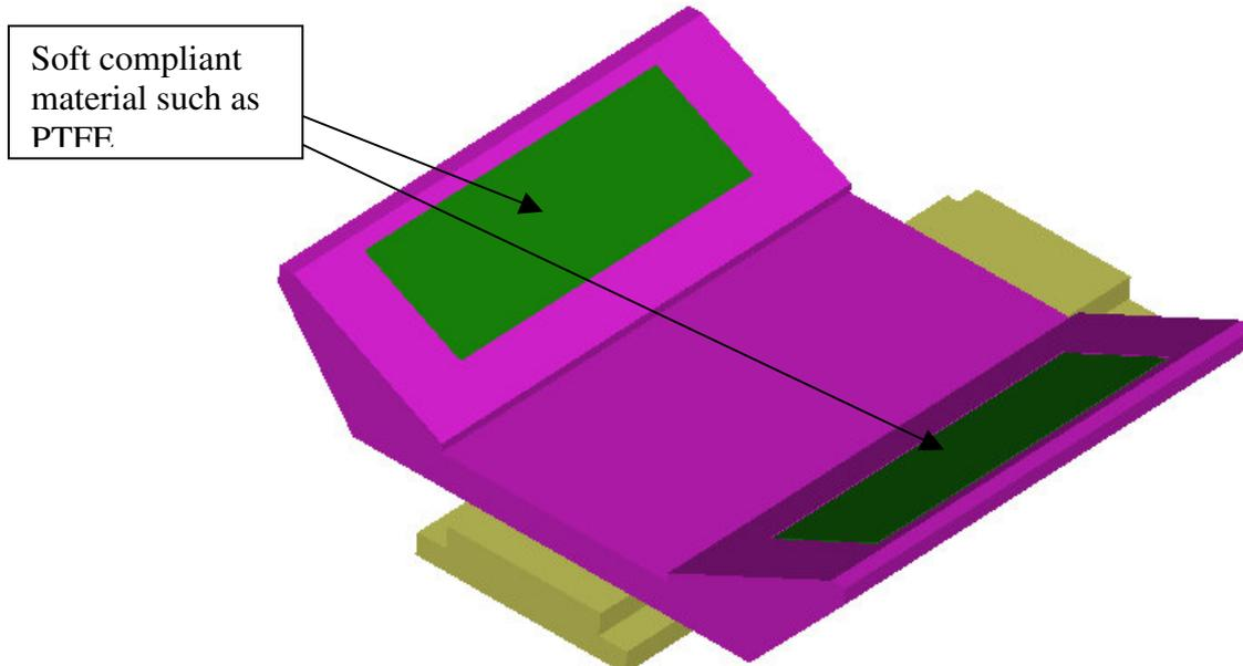
These pads are particularly important for the welding process, where it may be that a considerable amount of force is exerted on the masses, by the clamp, in order to get the necessary fibre stretch.
