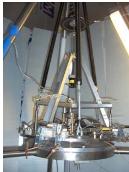
Scheme of the excitation system: 1) GAS blade; 2) Filter body; 3) Support spring; 4) Voice-coil; 5) Payload; 6) Rigid connector; 7) Accelerometer; 8) Rigid pyramidal connectors. All the apparatus was enclosed inside an isolation chamber to protect it by the air movement and to provide thermal isolation.
