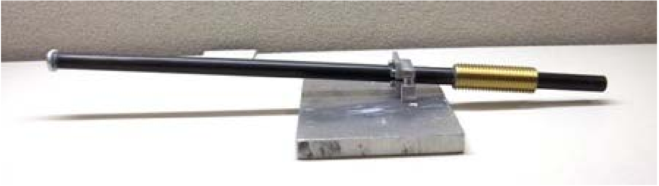
The carbon fiber wand constrained to the aluminum slab.
