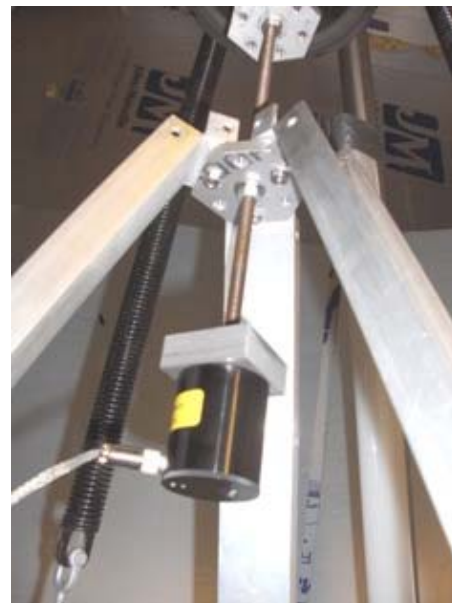
A piezoelectric accelerometer scheme (left). The TEAC accelerometer used for the input (right).
