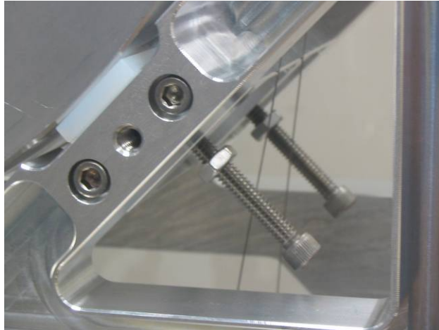
Fig 3. Teflon pads and safety stops
