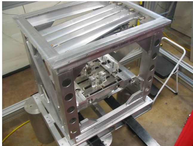
Fig 5. Upper structure with top stage and top mass installed, shown on aluminum palette supported on 3 table legs for ergonomic assembly. (CT)
