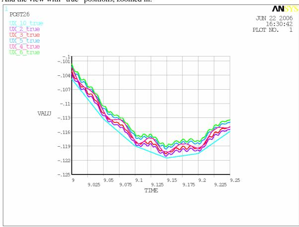
Hmm – how significant is it that the bounces seem to coincide with the (0.05 sec) discretization of the displacement data? To test this I would need to make a smoothed version of the displacement data with finer granularity.
