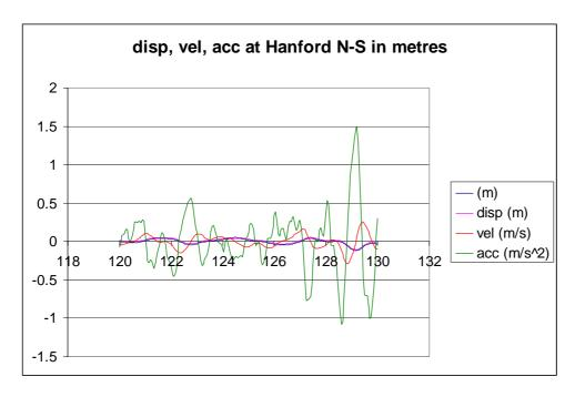
(NOTE that the max displacement is ~120 mm!)
