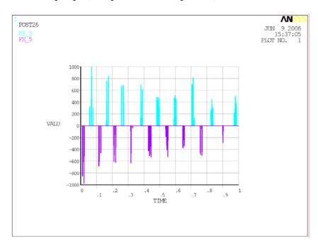
Hmmmm. Although the exact form of the contact is different each time, the magnitude of the forces is not changing. So settle on 5,000 substeps per second and press on to a full solution for the ten seconds.
