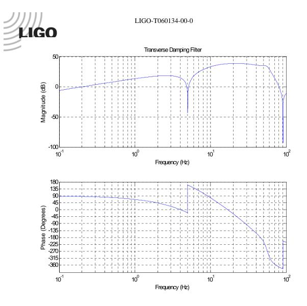
The standard filter uses a zero at 0 Hz and two poles at 16 Hz. Some of the DOFs have an additional gain between 0.5 and 5 in order to improve damping or stability. The transverse filter uses a zero at 0 Hz, a notch at 5 Hz, 3 poles at 10 Hz, 1 pole at 15 Hz, and an elliptical filter that begins rolling off the gain at 56 Hz. The latter filter is not used on the main chain.
