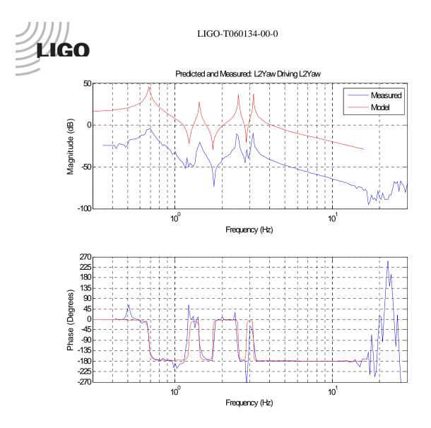
Again, the greatest discrepancies are in pitch. L1 pitch has a zero at 6.3 Hz, which coincides with the first zero at L2 longitudinal. The 1.6 Hz peak coincides with the 1.6 Hz peak from the local pitch DOF. The first L2 Pitch mode occurs at a greater frequency as well.
