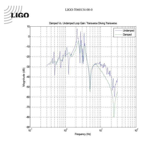
The lowest longitudinal mode does not show much damping here but the controller gain has been adjusted since this data was taken. There was not enough time to include the new data but damping is now much more significant. The roll damping has been adjusted as well and also has more damping then shown.
