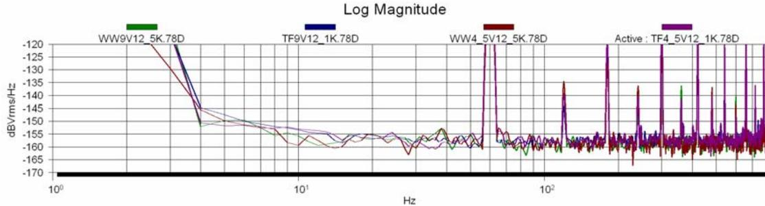
As can be seen from the plots, excess noise is not observed for either applied voltage.
