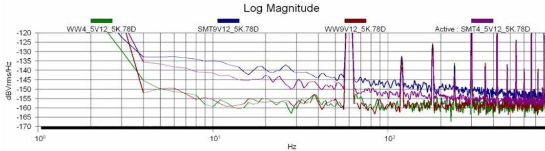
The measurement results for the 1Kohm wirewound and thick film SMT resistors are shown in curves below.
