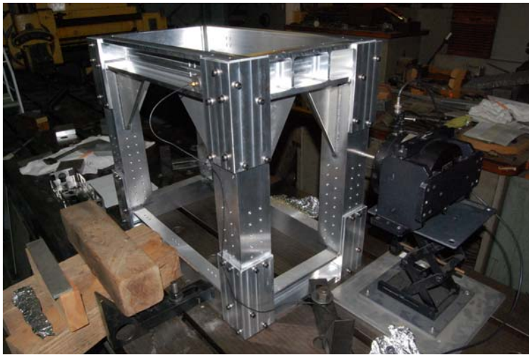
Figure 1: set-up for first set of measurements. Note that the scissors table under the driver was replaced by heavy steel blocks in later measurements.
