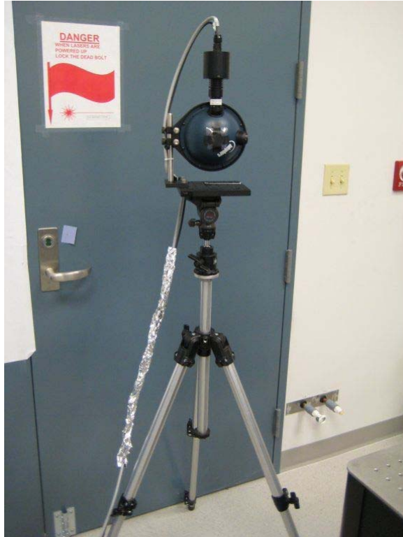
Figure 1 Working standard mounted on tripod for in-chamber measurement.
