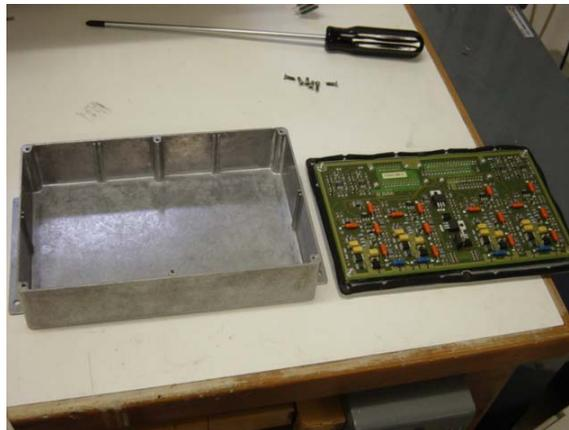
The picture below shows the TOP Coil Driver chassis with the top cover removed.
