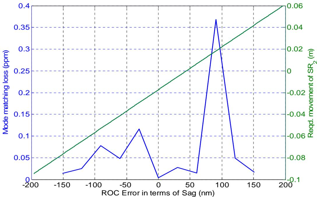
Fig. 7; Equivalent of Fig. 6 assuming that the errors are common mode and the compensation mechanism is motion of SR<sub>2</sub>.
