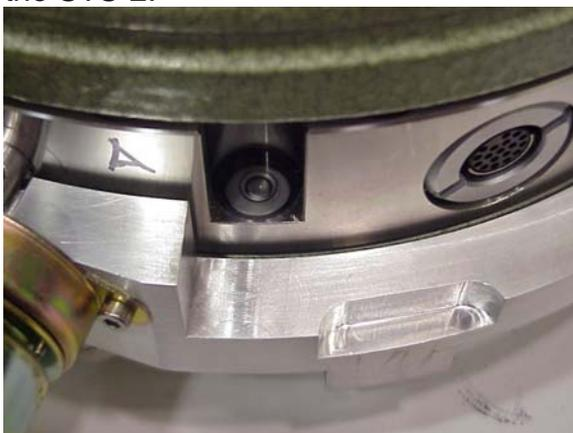
After leveling the STS-2, set in place the Foot Clamp (20007793-1) and Cross Bar (20007794-1) being careful not to ground or interfere with the motor wires. Make sure that the Cross bar protrusion is set into the indentation in the foot. Then install the  $\frac{1}{4}$ -28x 1  $\frac{1}{2}$  bolts (C-2824-NA) and vented washers (WFV-25). Torque to 68oz in. The wires will need to be positioned on top of the Foot after it is clamped.
