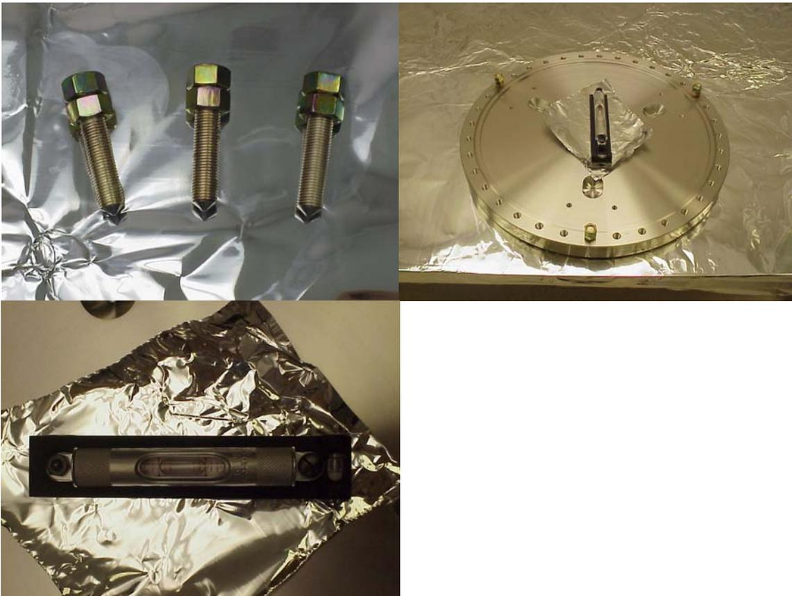
The locking nut (20007792-1) can be installed (with the boss facing the bottom of the STS-2) onto the 3 studs on the bottom of the STS-2, run them all the way up. Now install the Kinematic feet (20007791-1) on to the studs as well, run them up about half way through the foot. Caution here if you run them all the way up they will clip the bevel on the bottom of the STS-2.
