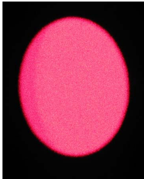
Figure 5: Laser speckle at the input port of the gold standard integrating sphere when illuminated by a laser pointer
