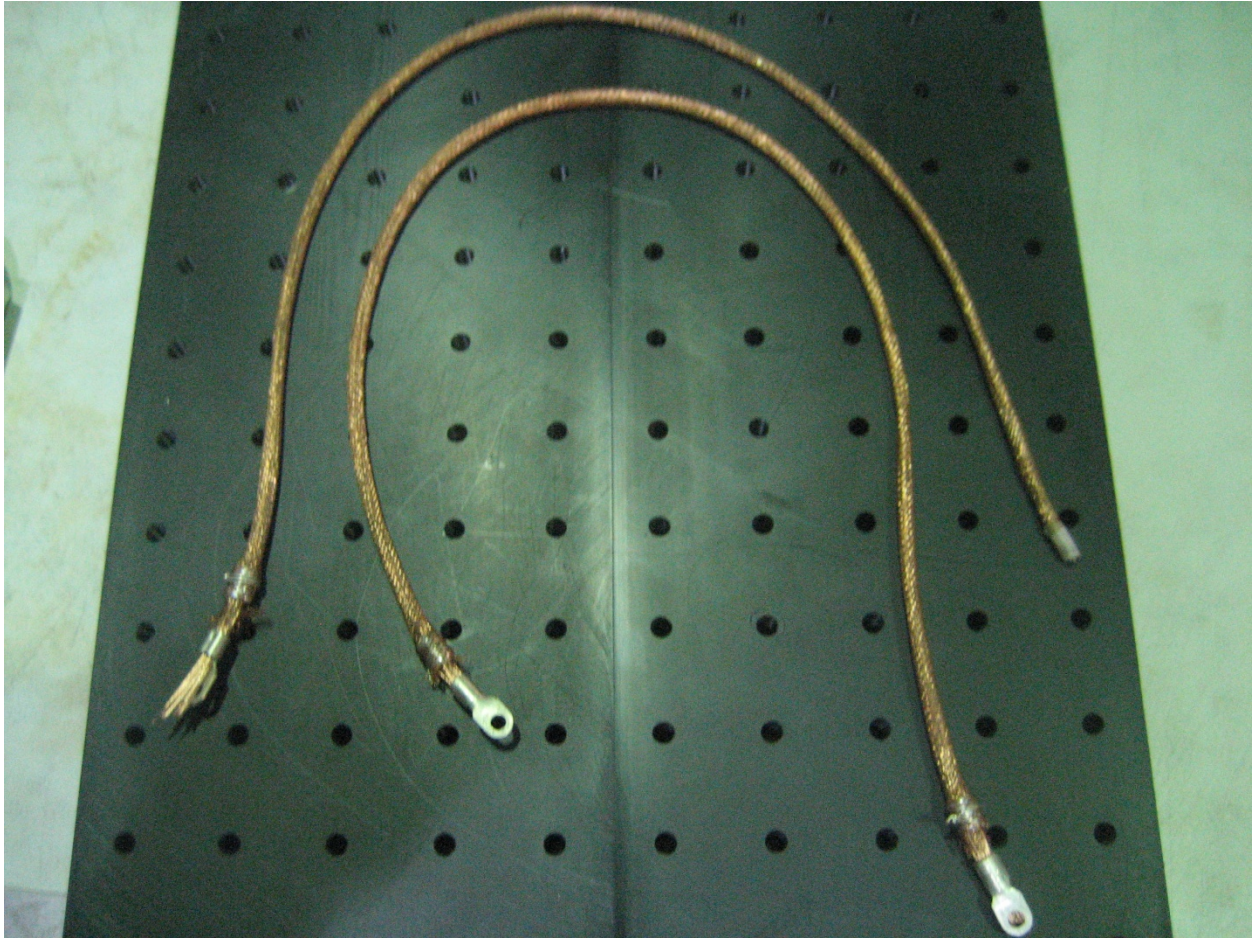
Figure 4. The cabling used in our experiments. Two such cablings are used in the OMC double pendulum suspension.
