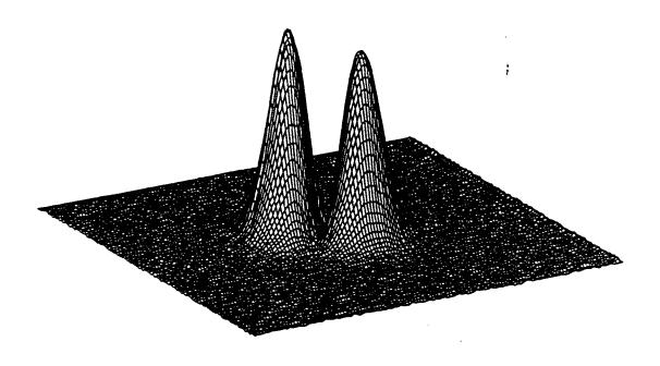
Figure 1. Transmitted light intensity from stationary interferometer cavity resonating in  $\text{TEM}_{01}$  mode.
