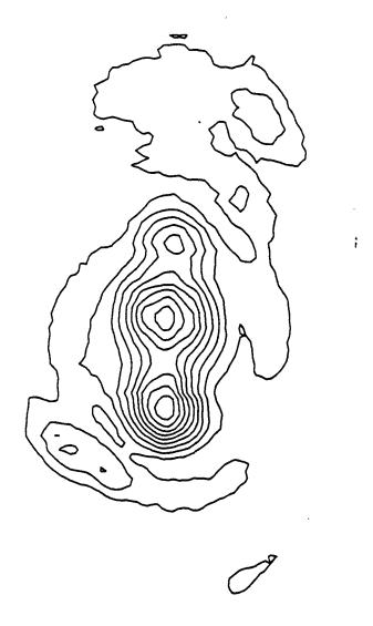
Figure 2. Intensity at dark fringe output of stationary interferometer.
