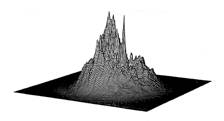
Dark fringe for beam at x=0,y=0,w=2 cm
