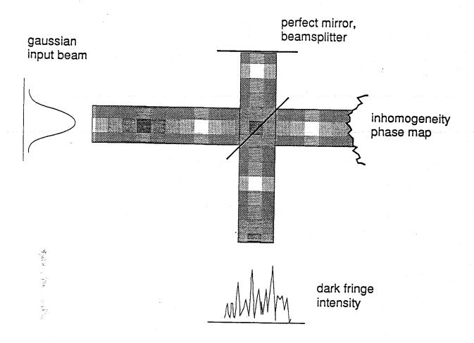
Setup for calculation: Michelson interferometer
