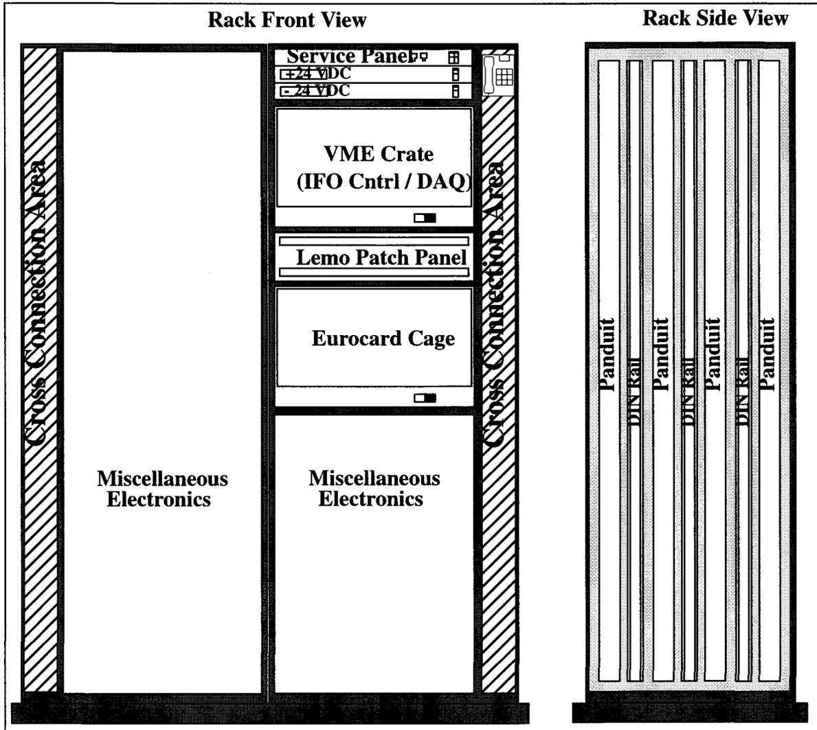
Figure 5: CDS Standard Front End Rack Assembly (LVEA)
