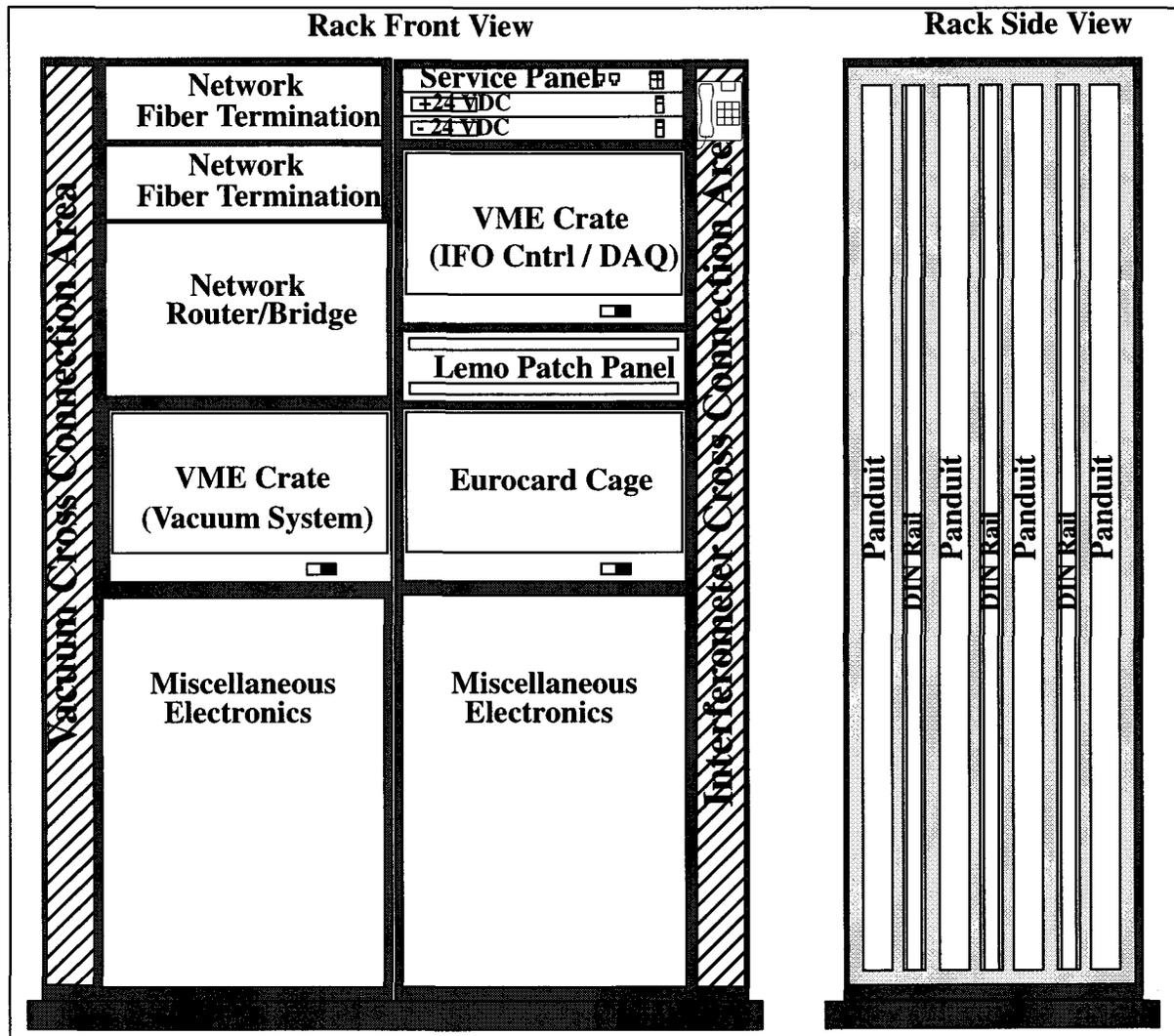
Figure 6: Standard Rack Layout (Mid and End Stations)
