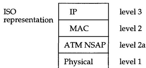
The introduction of the new Media Access (MAC) layer does not fit within the standard ISO representation, but this is hardly surprising since we effectively have a "network in a network".
