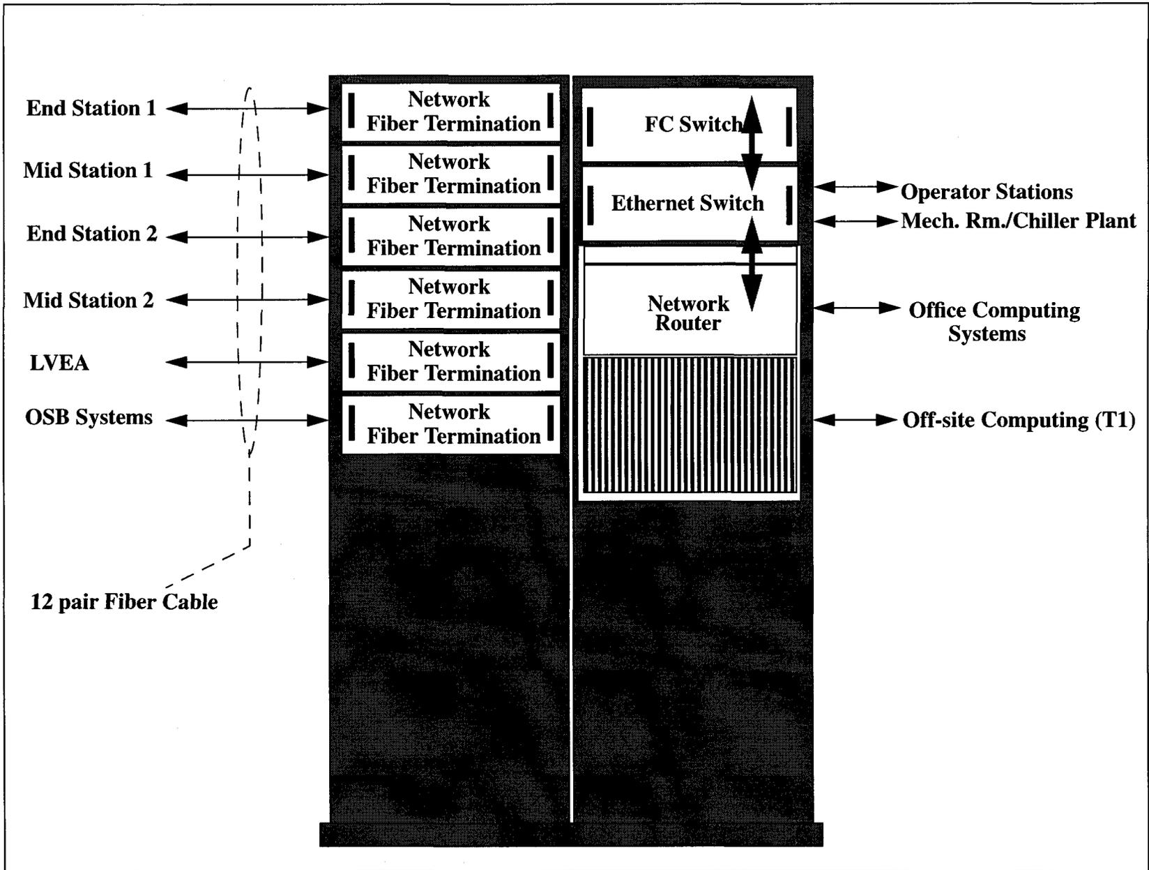
Figure 12: Network Rack Layout (OSB Computer/Mass Storage Room)
