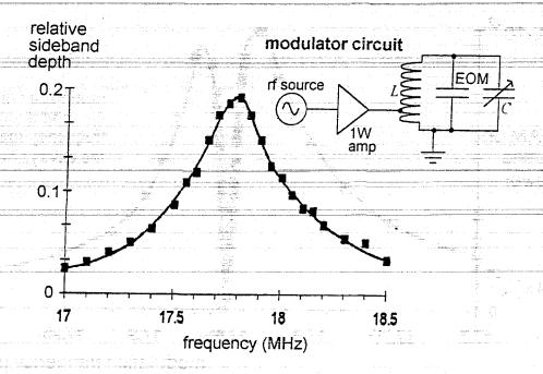
Figure 2: The circuit used to apply modulation sidebands on the light with adjustable frequency  $f_1$ . The linewidth of the prototype modecleaner cavity is only  $20\,\mathrm{kHz}$ , hence in view of the resonance curve of the modulator circuit shown here we may deduce that the variation of applied sideband height is slight over several cavity linewidths.
