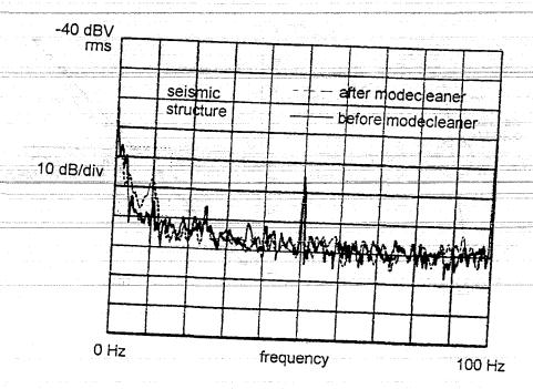
Figure 6: Traces showing the photodiode signal demodulated at  $f_1$  measured for the light entering and exiting the modecleaner cavity. With a greater span we observed that by several hundred Hz the backgrounds of both traces tend to the measurement shot noise level for the light power used (25 mW); around 10 dB lower than the background level at 100 Hz.
