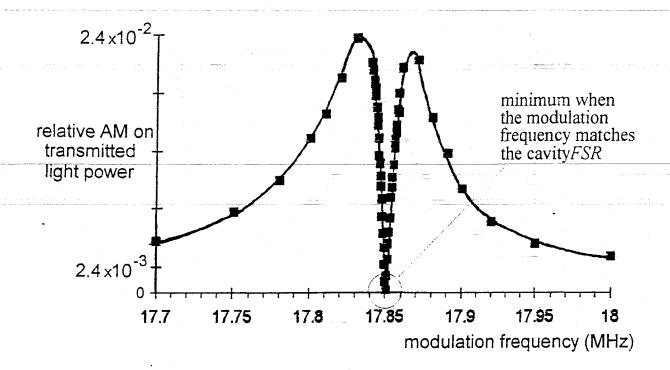
Figure 3: The amplitude modulation of the transmitted light power as the sideband frequency is varied through the modecleaner cavity FSR.
