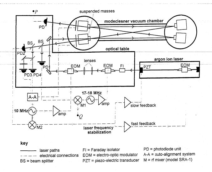
Figure 1: Experimental arrangement of the apparatus used to investigate the process of passing modulation sidebands through a modecleaner cavity.
