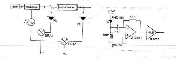
Figure 5: A simplified diagram showing the experimental arrangement to investigate the light noise demodulated with respect to  $f_1$ . The signals to be spectrum analysed at A and B are those associated with the light after and before the modecleaner.
