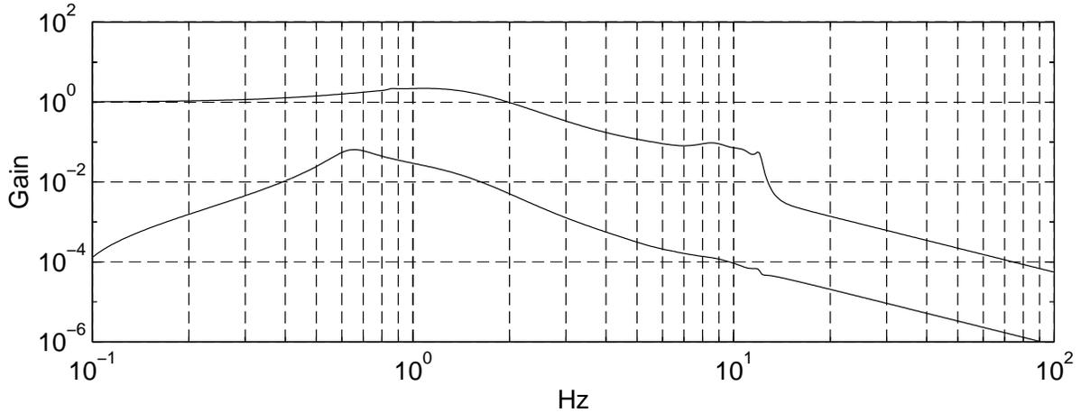
**Figure 3: Transfer function from the horizontal displacement of the suspension position to the cavity length variation via the horizontal motion (Upper) and via the pitch angle change with assumed  $d$  of 1 cm (Lower).**
