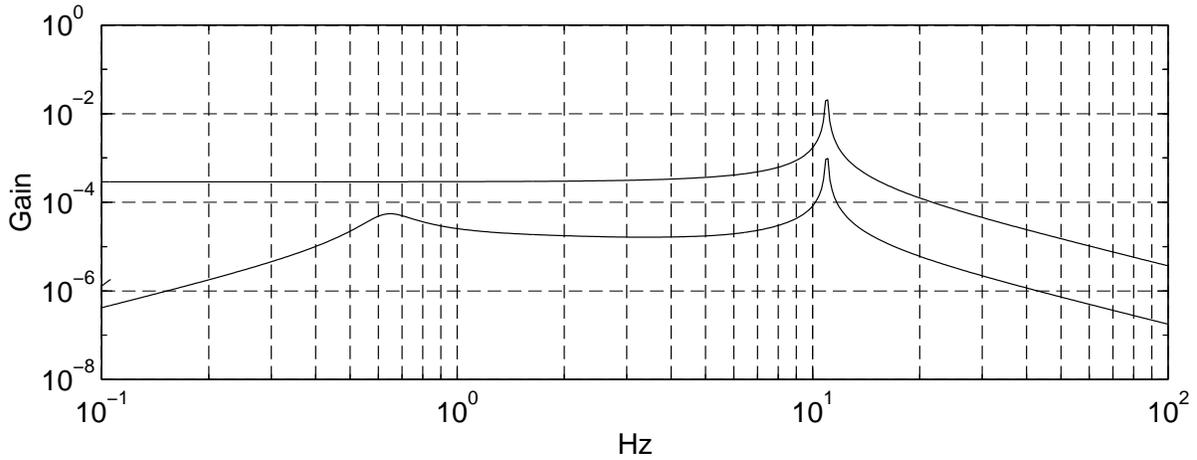
**Figure 6: Transfer function from the vertical displacement of the suspension position to the cavity length change via the vertical motion coupling with the earth's curvature (Upper) via the pitch angle change with assumed  $d$  of 1 cm (Lower).**
