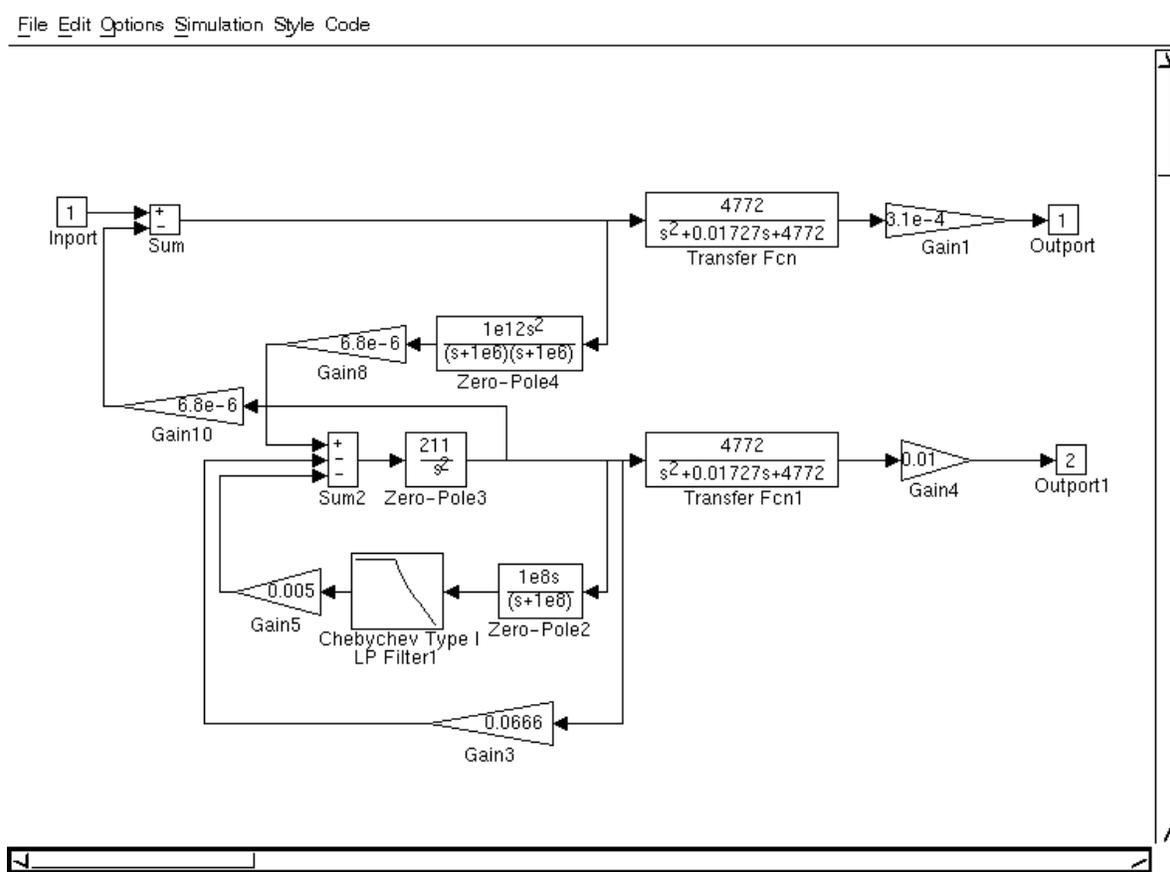
**Figure 5: Block diagram of the pendulum system with vertical motion of the suspension point.**
