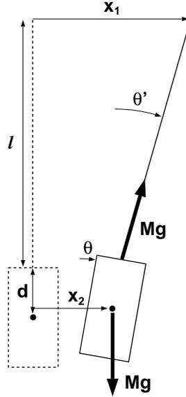
**Figure 1: Response of the pendulum system to the horizontal motion of the suspension point.**
