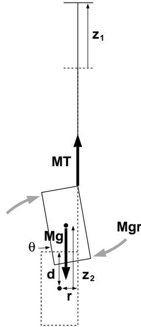
**Figure 4: Response of the pendulum system to the vertical motion of the suspension point.**
