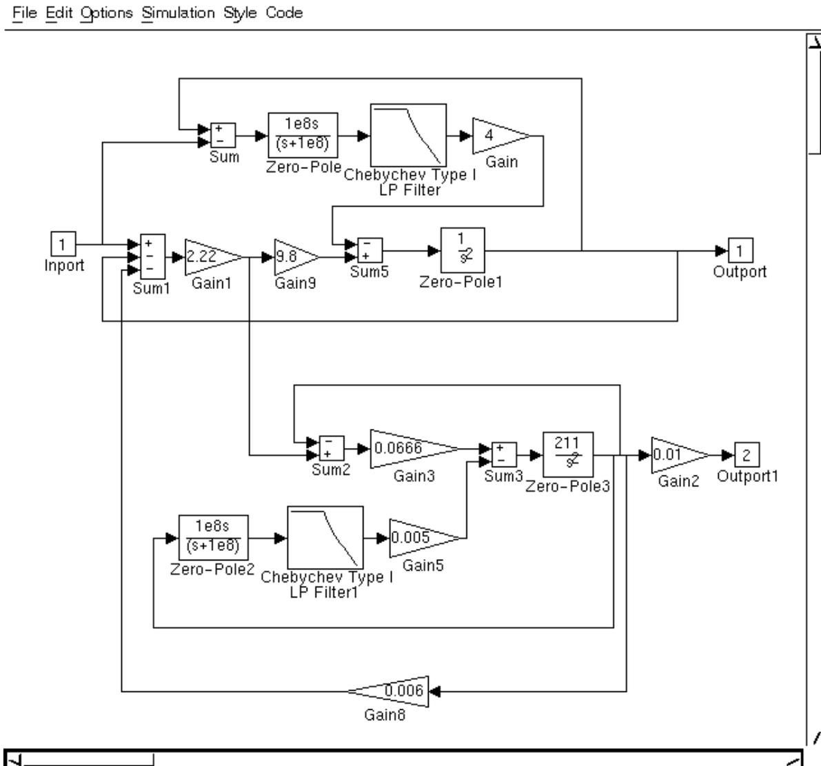
**Figure 2: Block diagram reflecting the equation of motion of the pendulum system with horizontal motion of the suspension point.**
