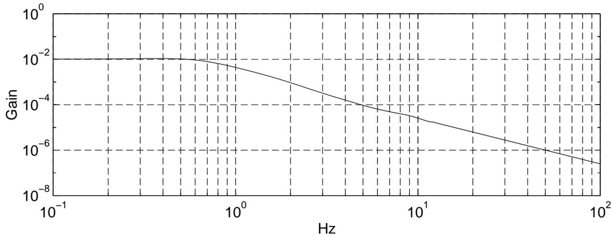
**Figure 7: Transfer function from the yaw angle of the suspension point to the cavity length change via the yaw angle change with assumed  $d$  of 1 cm.**
