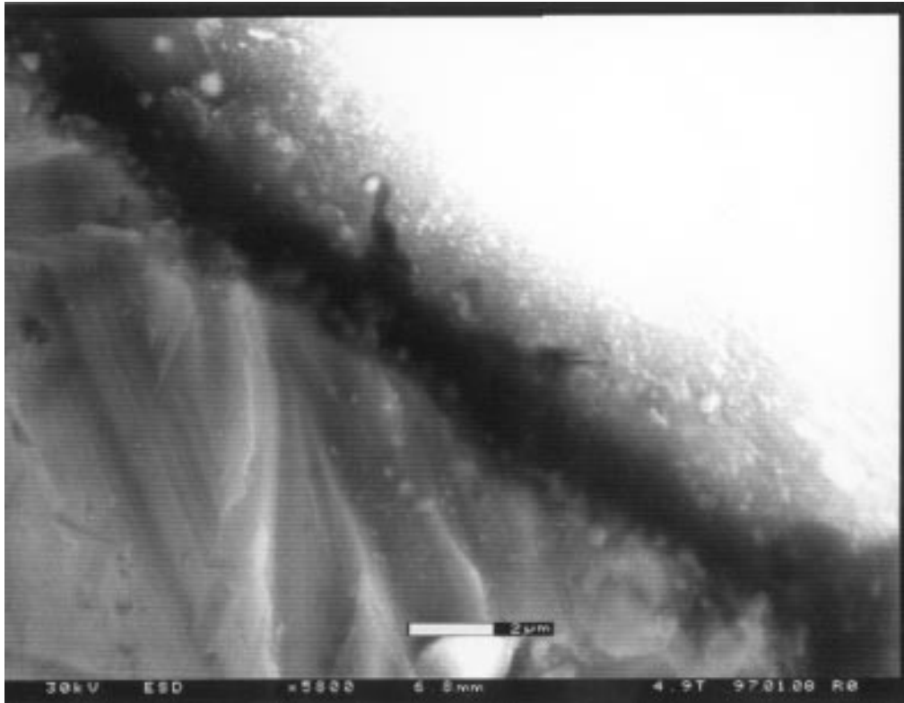
Figure 2 Scanning Electron Microscope picture of cross-section of thin non-shedding baffle.
