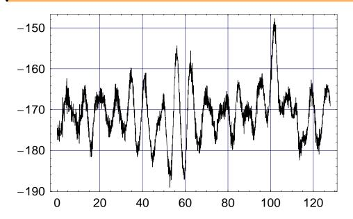
After subtracting the mean value from the time series we compute the Fourier series and estimate the power spectral density (no windowing function)
