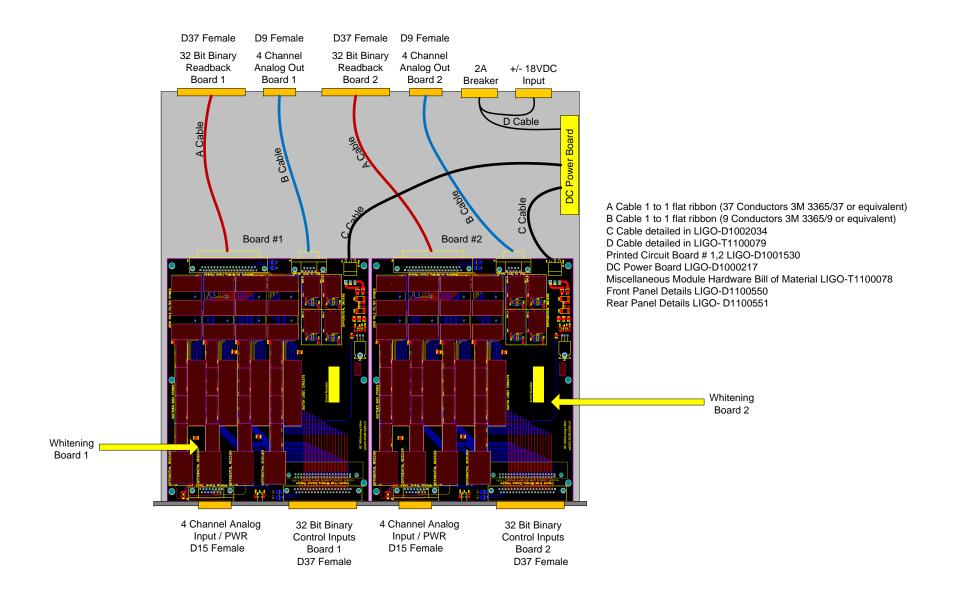
Dual Optical Lever 8 Channel Whitening Chassis
