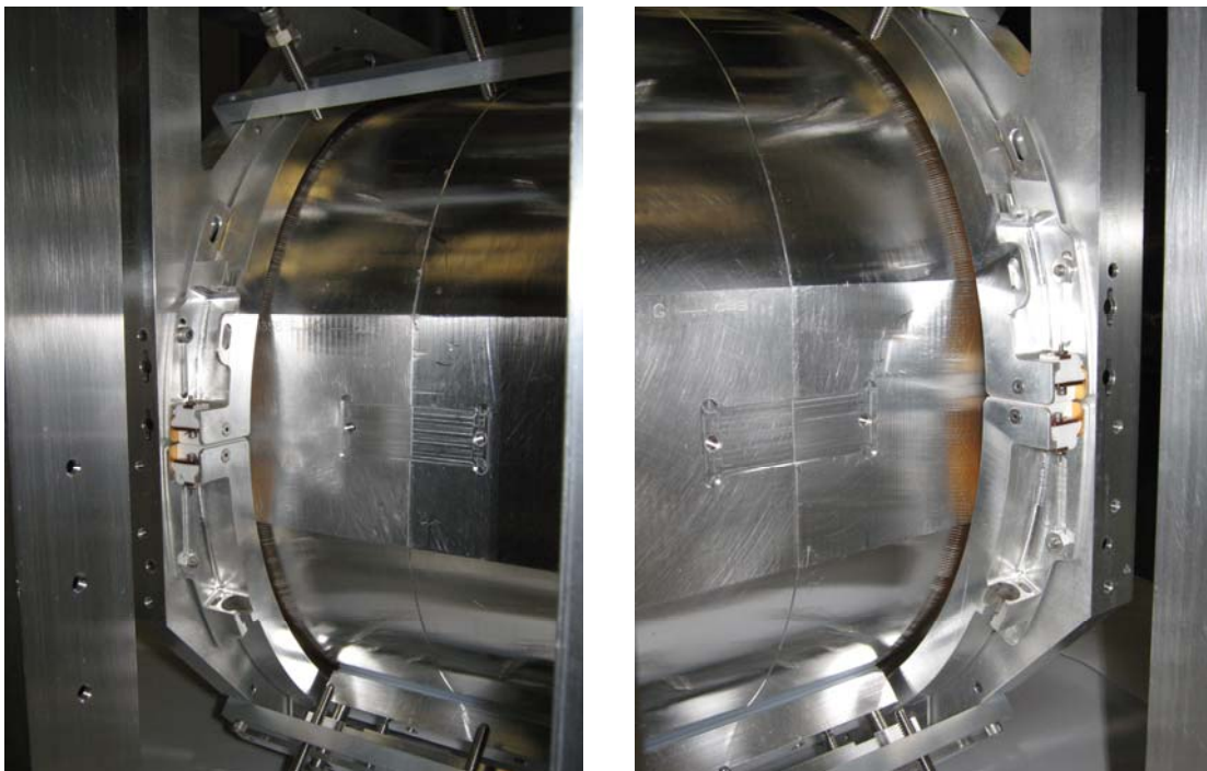
Figure 2: Final Design Prototype Assemblies (D1001838-v1 & D1001895-v1) integrated with the aLIGO Production Quad Structure.
