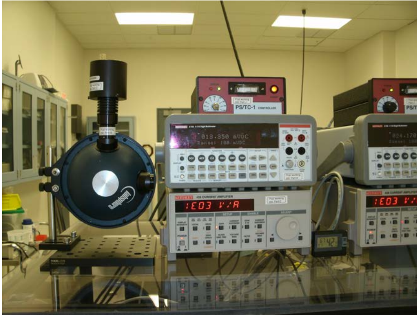
Figure 29 – eLIGO Working Standard power sensor including the integrating sphere, photo-receiver module, fast current amplifier, digital multimeter, and power supply/thermo-electric cooler controller.
