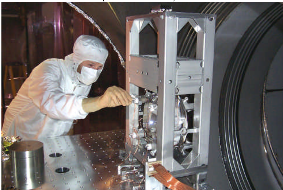
FIGURE 3. Installation of a suspension tower assembly within the interferometer vacuum.
