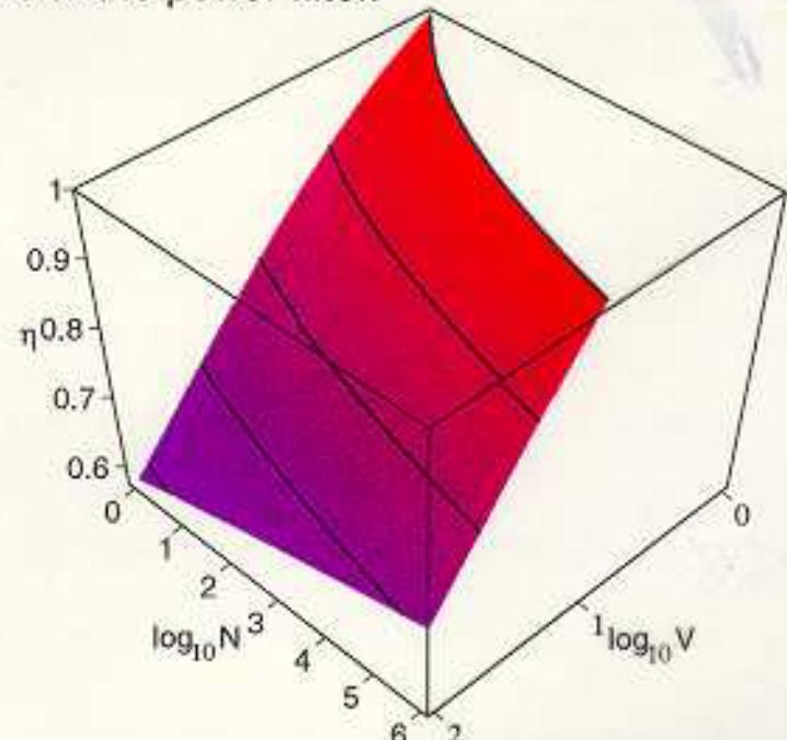
If the number of filters in the bank is large and the time-frequency volume is small, the power filter is almost as effective as a bank of matched filters.
