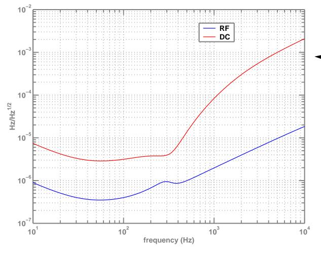
Requirement for frequency noise to be 10x below Bench strain sensitivity
