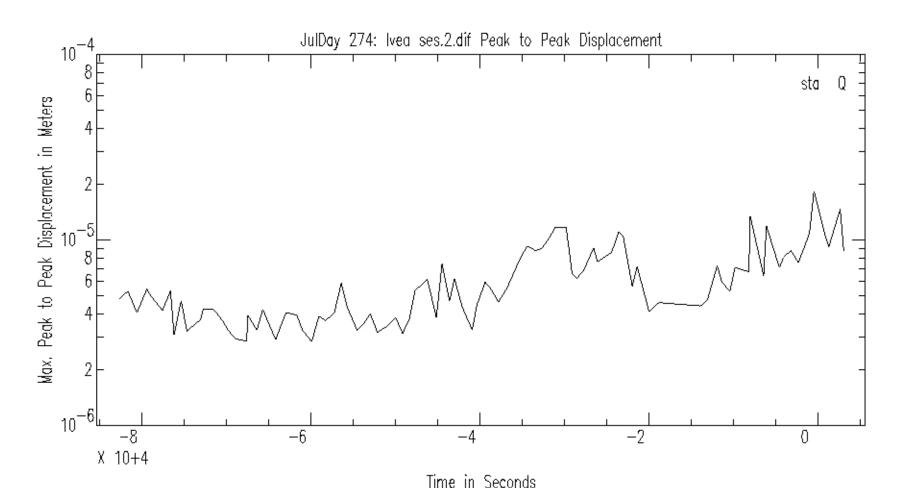
Bandpass .05 - .2 (Micro\_Seismic)
