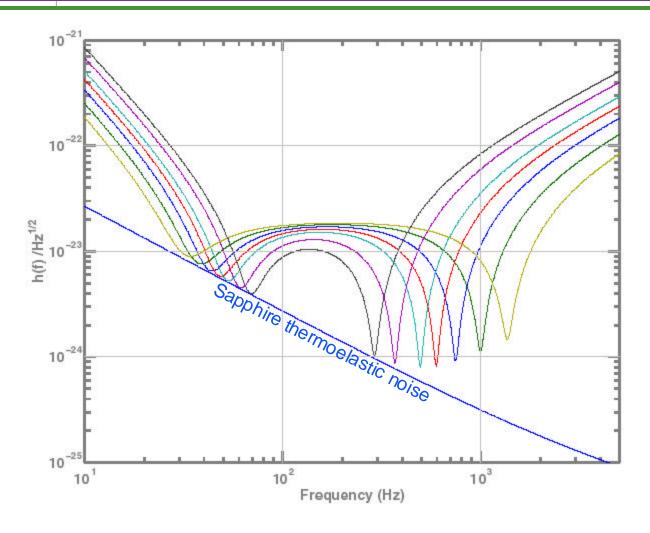
Example tuning curves for a fixed transmission signal recycling mirror
