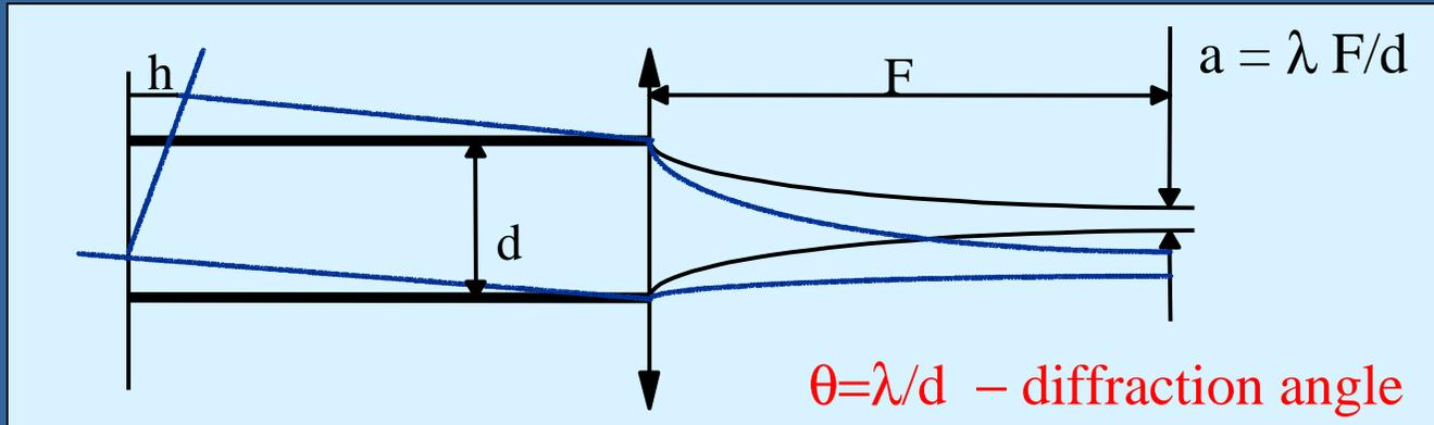
In linear electrodynamics the major limitation to measure wave front deviations angles comes from a finite size of the focal spot  $h = \lambda/20 \dots \lambda/50$  is achieved by an accurate measurement of the transverse beam distribution
