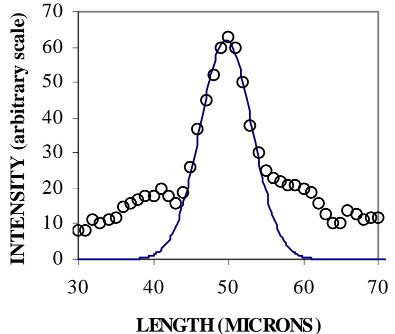
Of all the tested substances, the minimum size of a self-focusing point is in benzene, i.e. 5  $\mu\text{m}$  at the length of a nonlinear cell of 60 cm, which results in the precision of wave front inclination measurements  $\lambda/3000$ .
