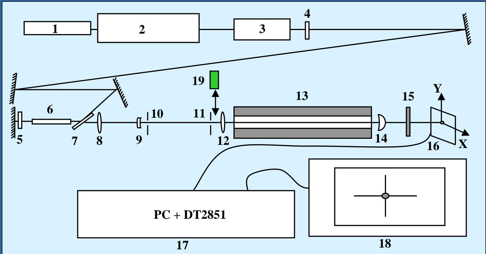
*1* – HeNe laser; *2* – Nd master oscillator; *3* – single pulse selector; *4* –  $\lambda/2$ ;
