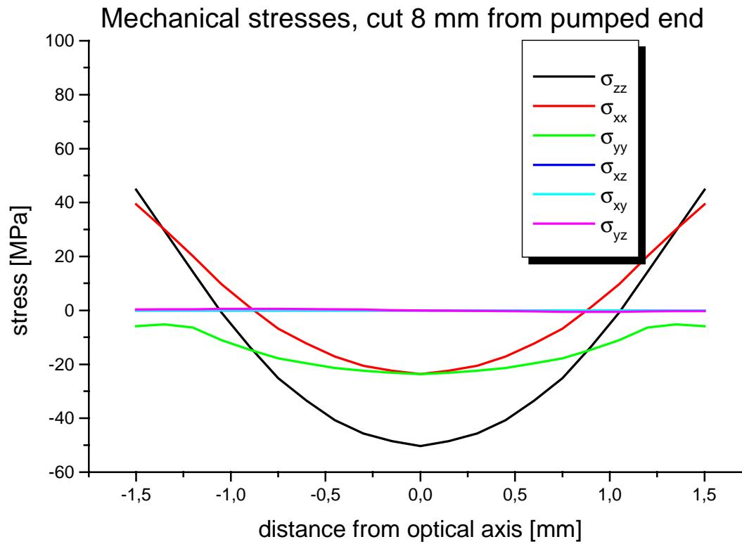
Well below fracture limit (130 thru 260 Mpa)
