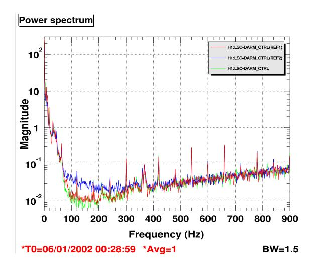
Fig. H1 power spectra before (red), during (blue), and after (green) the injection of a simulated stochastic background signal.
