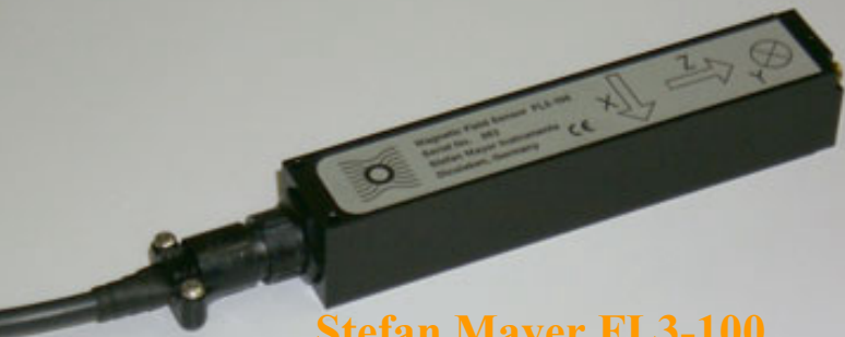
Stefan Mayer FL3-100 - triaxial fluxgate magnetometer - sensitive for f < 2 kHz - sample rate: 4096 Hz
