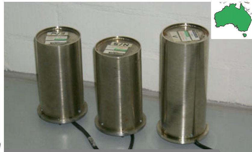
ACIGA: Guralp CMG 3 single-axis seismometers
