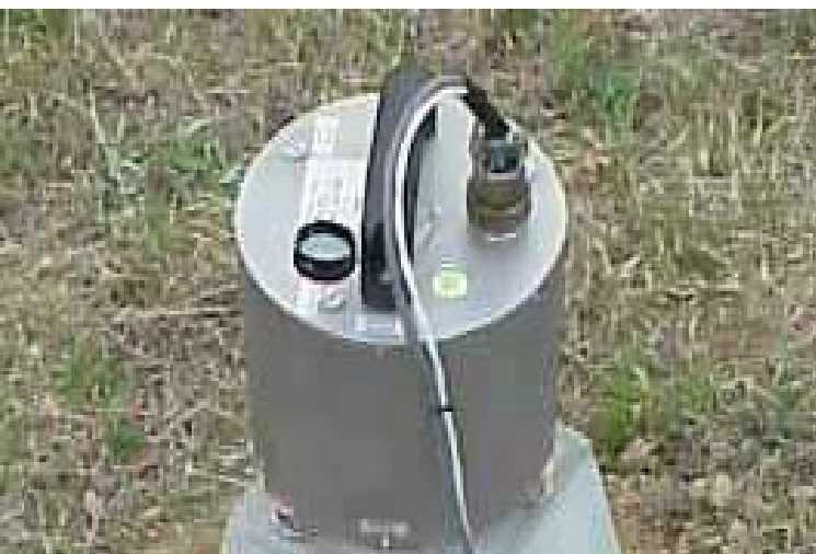
LIGO: Guralp CMG-40T triaxial seismometers
