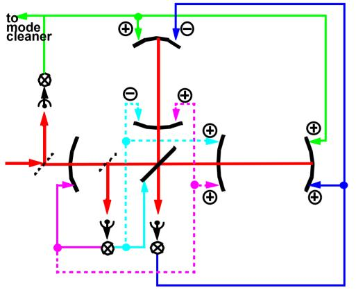
example: cavity length sensing & control topology
