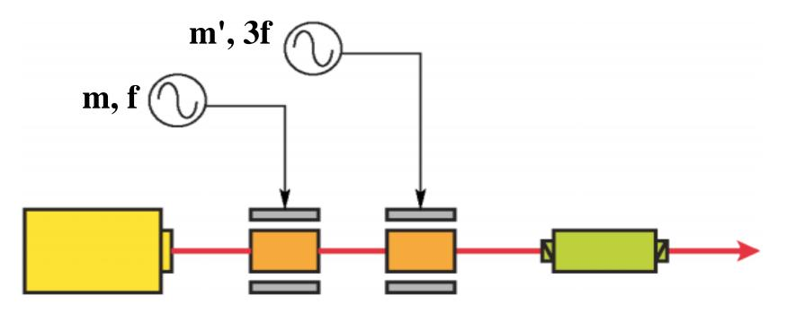
**Output** =  $(J_0 + iJ_1 \sin \omega t + J_2 \cos 2\omega t - iJ_3 \sin 3\omega t) (J_0' + iJ_1' \sin 3\omega t)$
