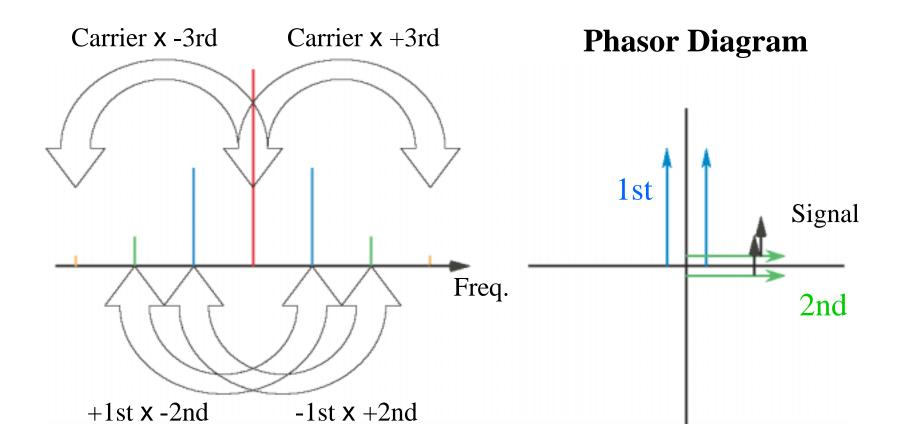
Beat signals of 1<sup>st</sup> and 2<sup>nd</sup> SB do not include L+/L- signals. But beat signals of carrier and 3<sup>rd</sup> SB are undesirable for THD.
