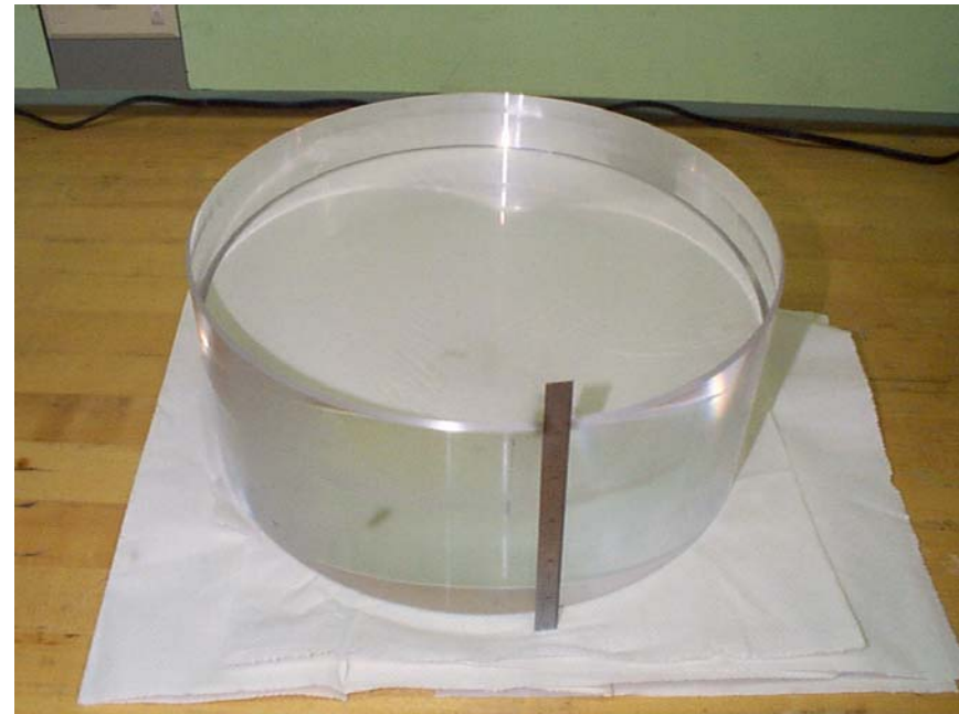
Full-size Advanced LIGO sapphire substrate
