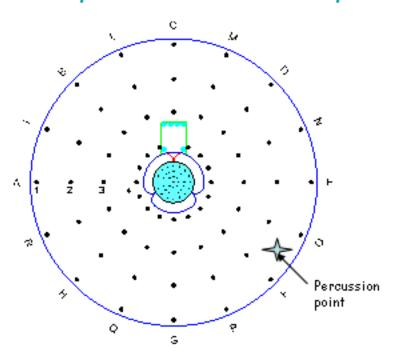
➤ We have used an impulsive technique by hitting the holder on an assigned point with a calibrated hammer and measured the induced displacement along the z direction, at each point of the map, with an accelerometer.
