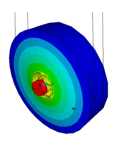
FEM Simulation of the First Symmetric Mode (5453 Hz)
