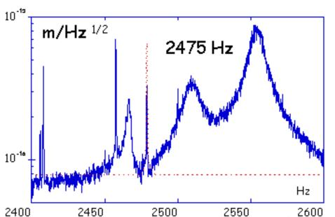
Comparison of the E4 displacements noise spectrum with the thermal noise contributions computed using the Lab measurements results.
