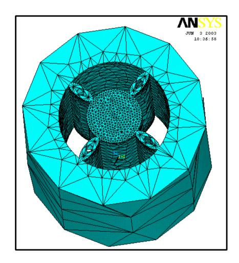
Schematic model integrating mechanical amplifiers and suspension system.
