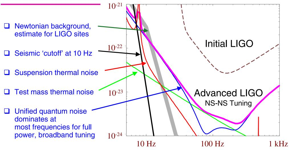
Advanced LIGO's Fabry-Perot Michelson Interferometer is a platform for currently envisaged enhancements to this detector architecture (e.g., flat-top beams; squeezing; Newtonian background suppression)
