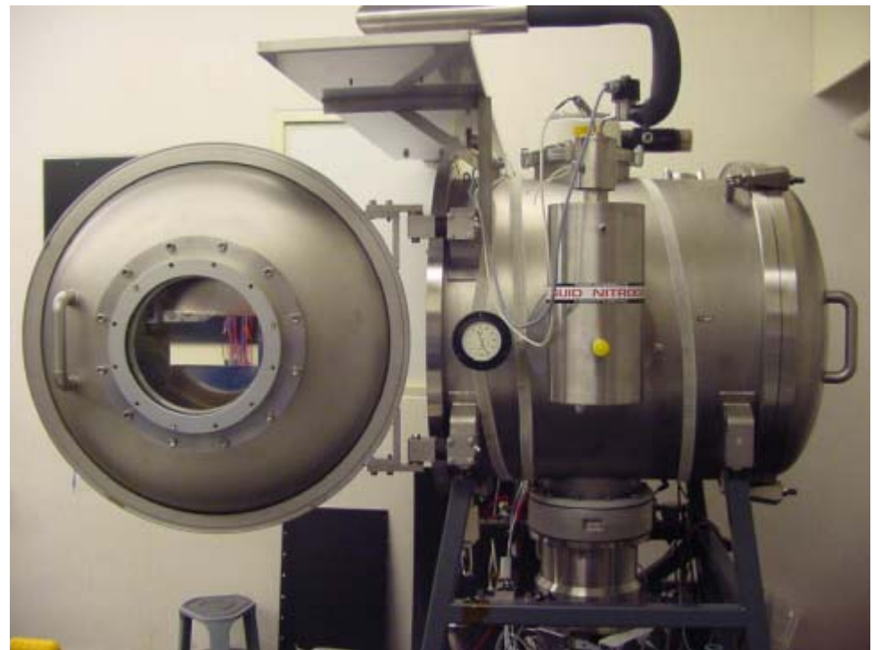
TNO test facility for thermal cycling
