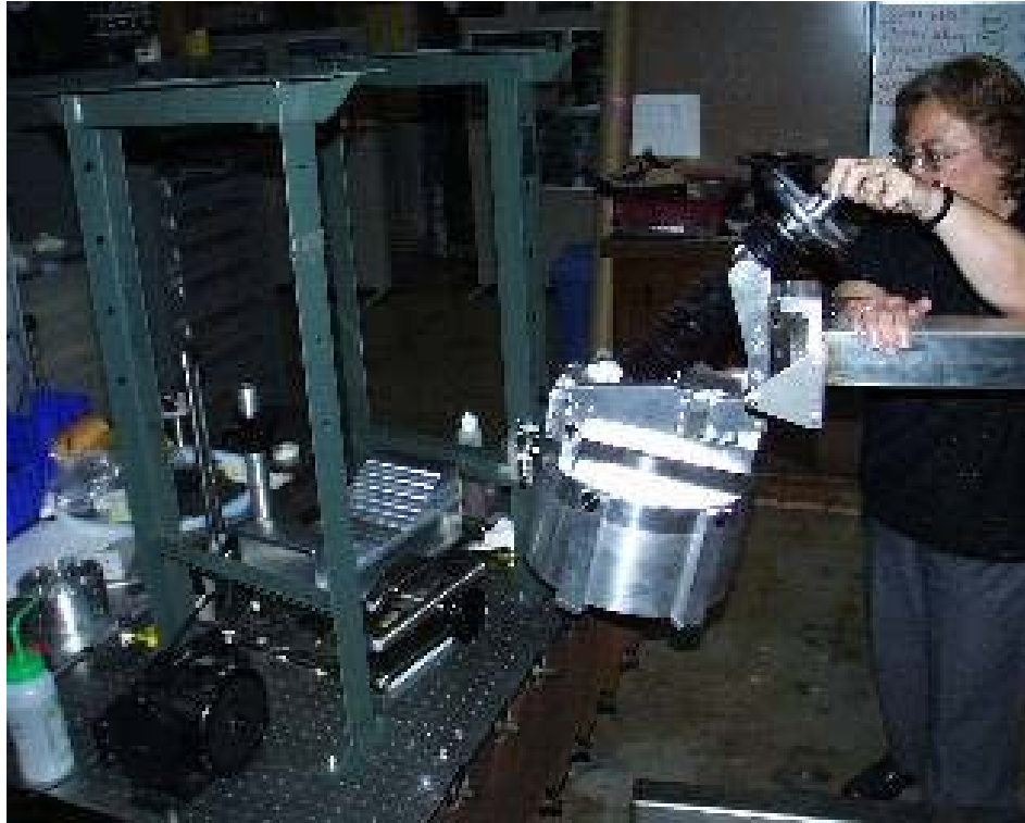
Dummy steel/aluminium mass, held by vacuum, being manoeuvred by ergonomic arm
