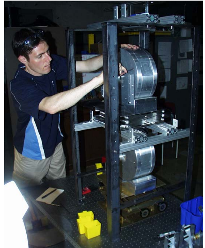
Prototype of penultimate and test mass being assembled at Caltech
