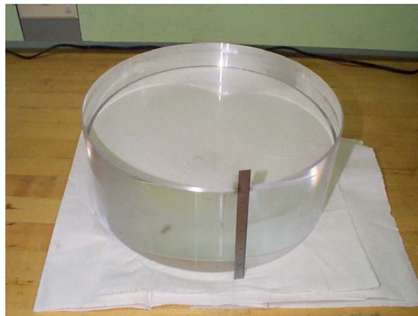
Full-size Advanced LIGO sapphire substrate
