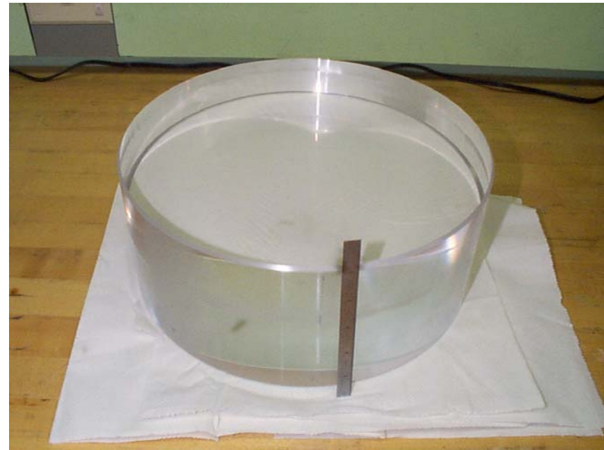
Full-size Advanced LIGO sapphire substrate
