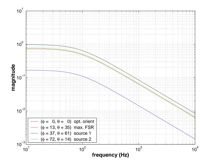
Sensitivity of the detector as a function of the source location: (*left*) at DC, (*right*) at FSR.
