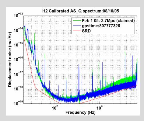
Note: The SRD curve (for the 4km), scaled properly for the 2km IFO, gives an inspiral range of 8.8 Mpc (vs. 14 Mpc for the 4k)
