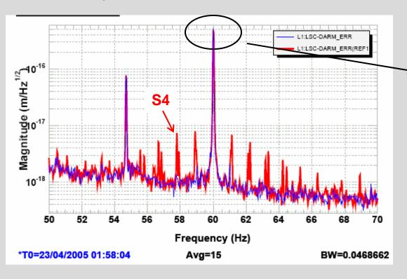
60 Hz peak later reduced by a factor of 2, by turning off a pipe heater in the Y end station; now 5x10<sup>-17</sup> m-rms
